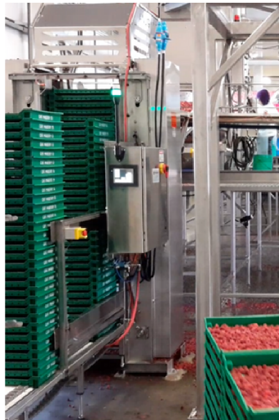
Lug dumping cycle time is fully adjustable-based on throughput requirements.
